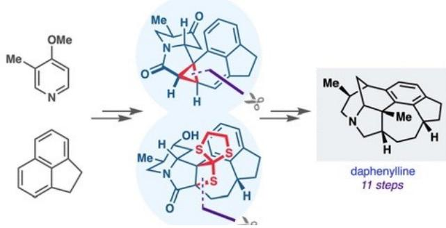
**Scheme 1. Total Synthesis of Daphenylline<sup>a</sup>**
